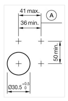
A = Action range of aligning pins
