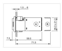
A = Screw terminal B = Plug-in terminal 6.3 mm x 0.8 mm
