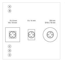
$\begin{array}{l} \mathsf{A} = \text{Terminals (rear side)} \\ \mathsf{B} = \text{Illuminated pushbutton} \\ \mathsf{C} = \mathsf{x} = \text{Contact No.} \\ \mathsf{D} = 2 = \text{Normally open} \\ \mathsf{E} = 4 = \text{Normally close} \end{array}$
