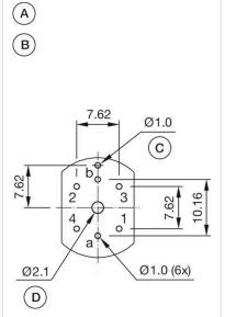
A = Axial socket B = Drilling-/occupancy plan (component side) C = non-metallic D = for central mounting with M2 screw, if desired
