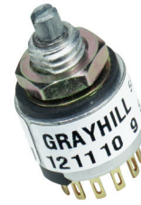
Screwdriver Slotted Shaft
