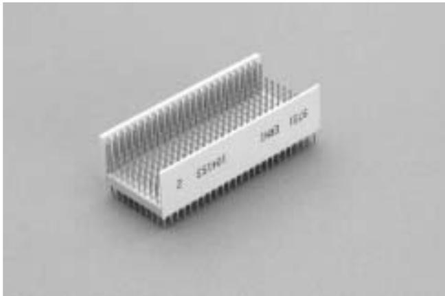
The ERmet type E vertical male connector provides 200 signal contacts and 50 ground shield contacts in an 8+2 row x 25 position fully loaded configuration. These connectors are also available in an 8+2 row x 22 positions and 8+2 row x 19 positions. With 15 different standard pin lengths to choose from, this is one of the most versatile connectors available. The connector is designed for gas tight pressfit installation.
