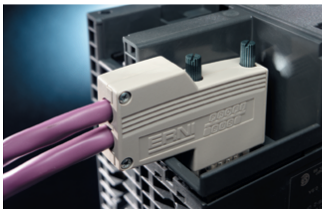
Integral T function, bus in, bus out
