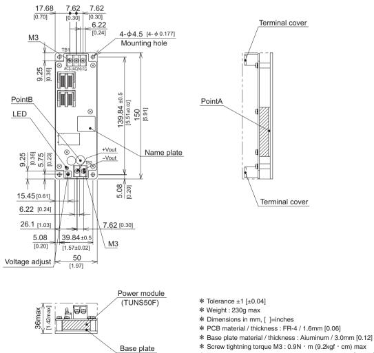
\* Please connect safety ground to the base plate in  $\phi$  4.5 [ $\phi$  0.177] hole.
