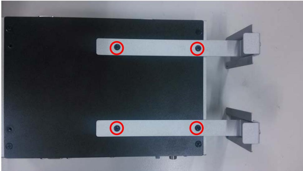
**Step 4 Depends on the thickness of the display or TV set, adjust the bracket and fasten the screws (per illustrated) in order to fit and hang on the TV panel, per illustrated**
