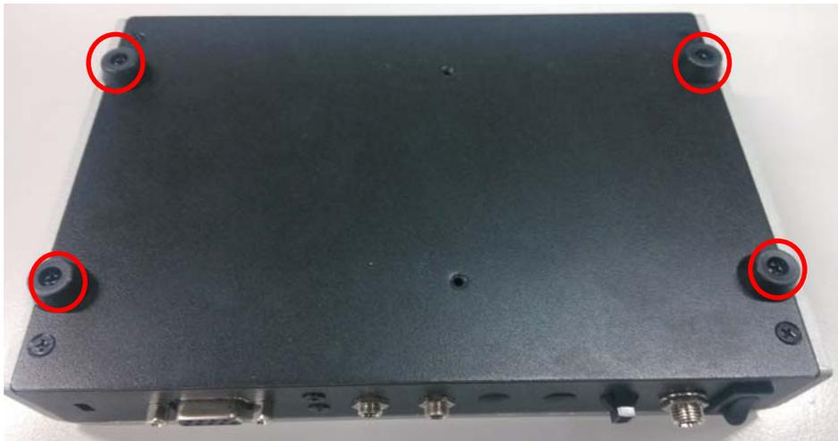
**Step 3 Put the DSB320-842 under TV rack kit and fasten screws per illustrated.**
