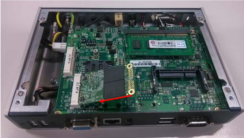
**Step 2** Push the module down, until it is firmly seated by locking two latches on the sides, and then fix the mSATA with screws with image illustrated
