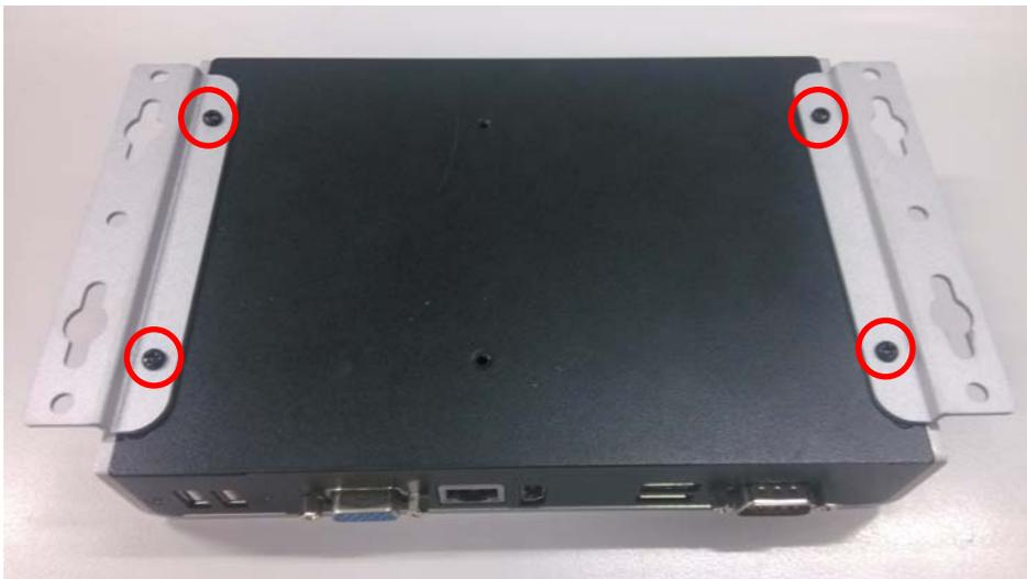
**Step 3** Fix the wall mount to the correct location, and fasten all screws.
