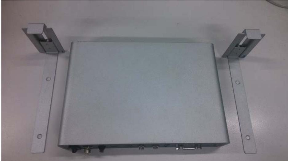
**Step 2 Loose the screw of four footpads at the bottom of DSB320-842, and remove footpad.**
