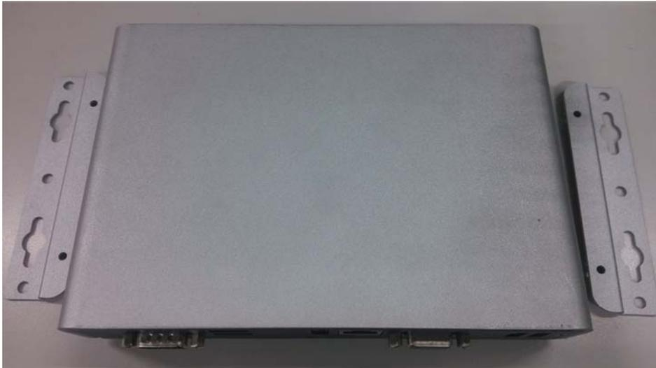
**Step 2 Fix the wall mount to the correct location, and fasten all screws.**
