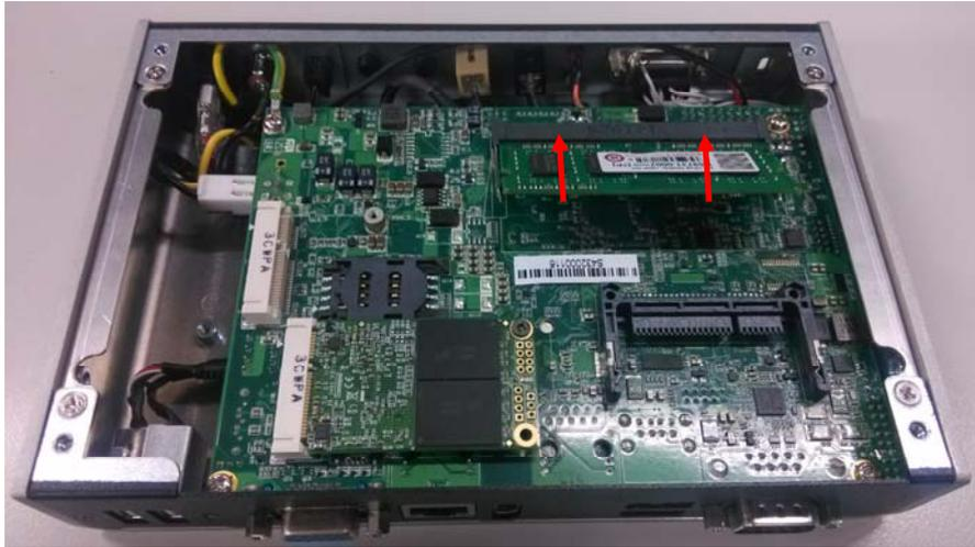
**Step 4** Push the module down, until it is firmly seated by locking two latches on the sides.
