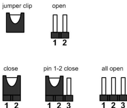
Properly configure jumper settings on the CAPA841/842 to meet your application purpose. Below you can find a summary table of all jumpers and onboard default settings.
