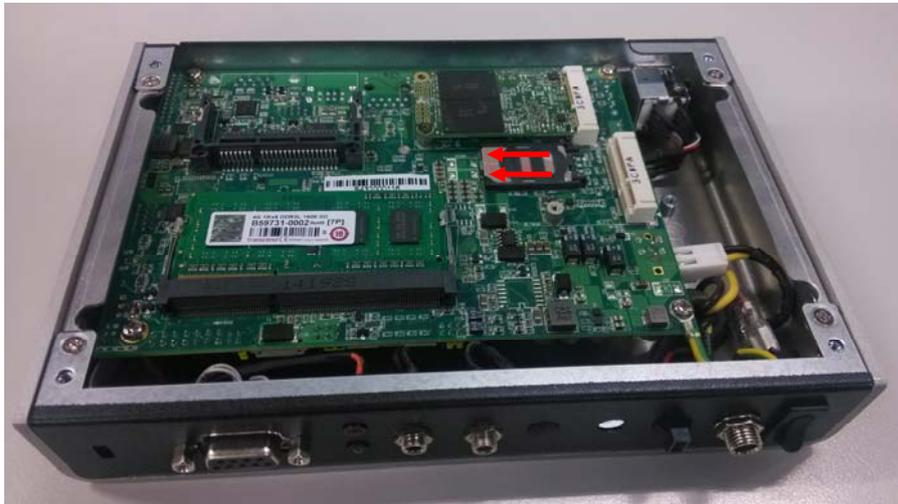
**Step 4** Install 3G module. Place the 3G module into the socket and press it firmly down, then affix the screws per illustrated.
