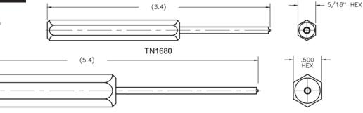
USING EITHER OF THE SPANNER WRENCHES SHOWN ABOVE, GUIDE SETS MAY BE REMOVED AND REPOSITIONED IN ANY OF THE 64 POLARIZING POSITIONS. REFER TO PAGE WA-18 FOR POLARIZATION CHART.
