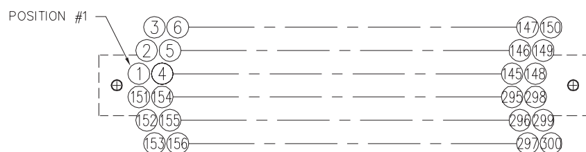
PIN IDENTIFICATION PATTERN VIEWED FROM MATING SIDE (EXAMPLE: 300 POSITION CONNECTOR)
