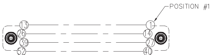
PIN IDENTIFICATION PATTERN (EXAMPLE: 52 POSITION CONNECTOR)
