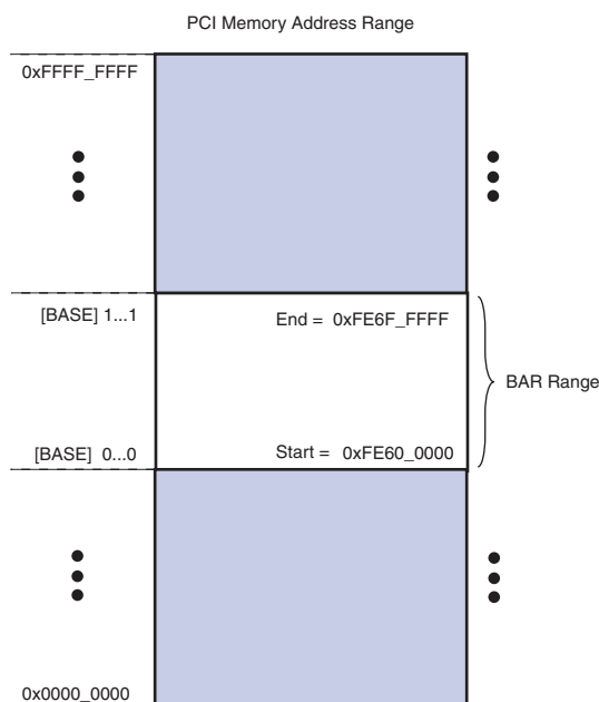
Figure 6–2. Pictorial View of the 32-Bit PCI BAR
