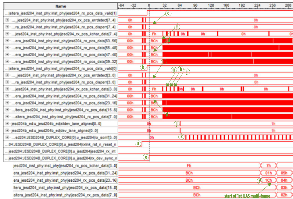
Figure 33. JESD204B Link Initialization
