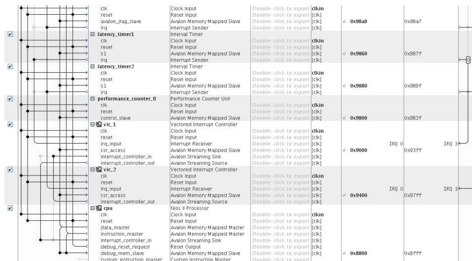
Figure 124. VIC Daisy-Chain Example
