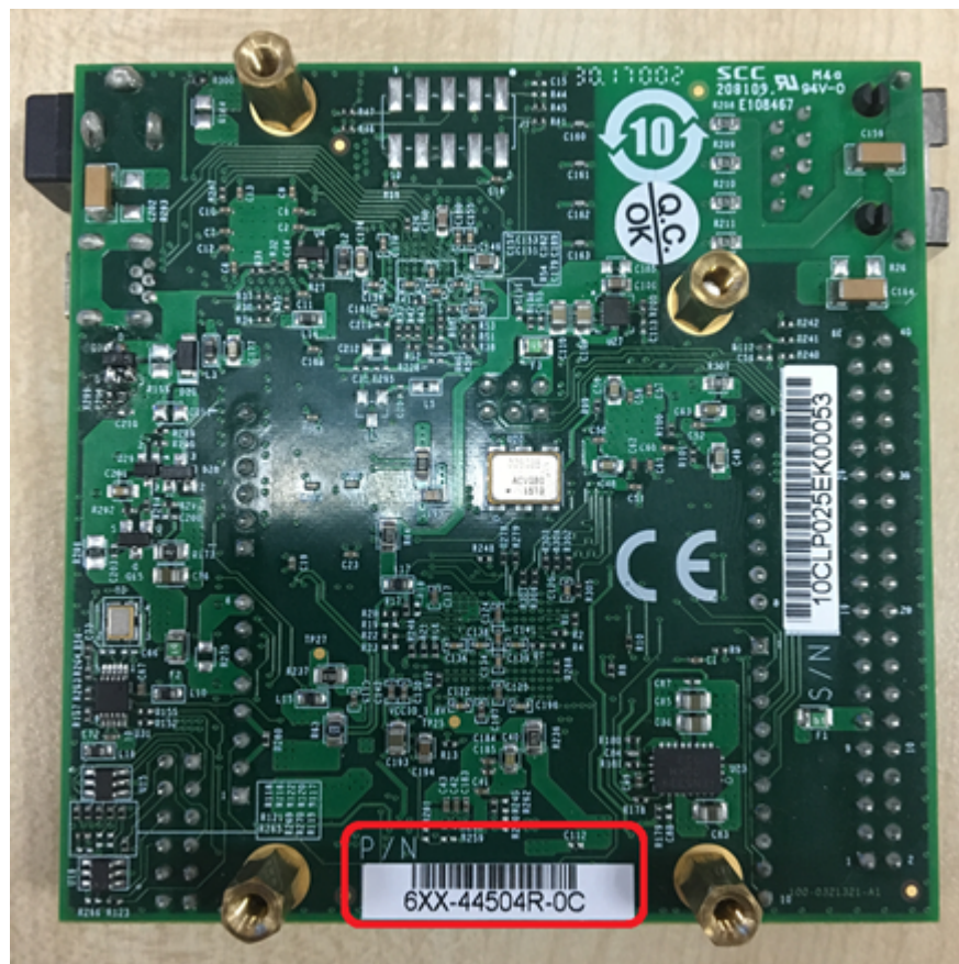
Figure 1. Intel Cyclone 10 LP Evaluation Board Part Number Label
