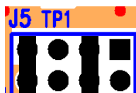
Figure 3: Shows the voltage selection jumpers
