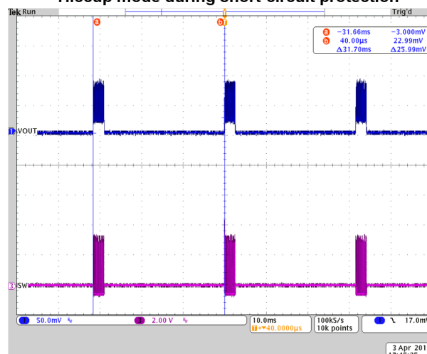
Hiccup mode during short-circuit protection
