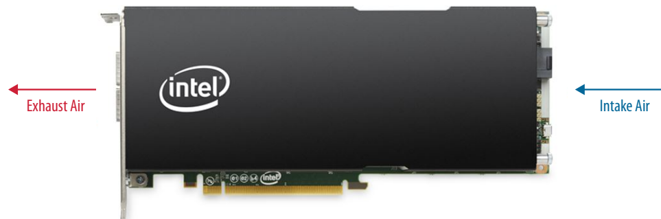
Figure 7. Intel FPGA PAC D5005 Airflow Pattern
