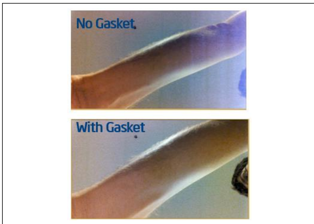
Figure 7-18. Example of Light Leakage Effects
