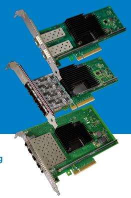
Dual and Quad-port 10GbE adapters with Hardware Optimization and Offloads for the Rapid Provisioning of Networks in an Agile Data Center
