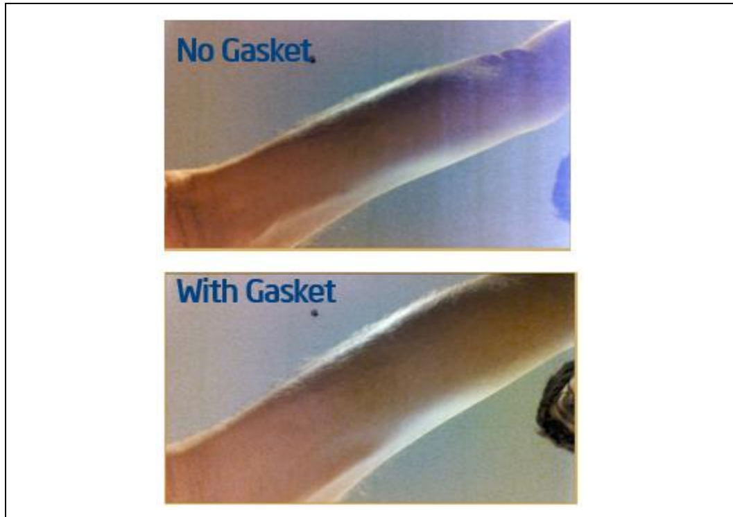
Figure 7-9. Example of Light Leakage Effects
