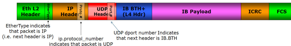
Figure A-41. RoCEv2 Packet Format
