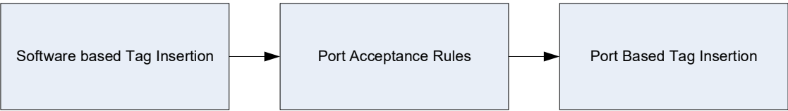
Figure 7-37. Transmit Tag Handling
