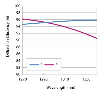
LightSmyth Technologies' transmission gratings are fabricated on fused silica substrates and robust dielectric films by state-of-the-art projection photolithography and reactive ion etch. These high fidelity semiconductor fabrication methods enable precise realization of sophisticated proprietary grating designs that provide diffraction efficiency close to 100% and line spacing control to 1 part per million.
