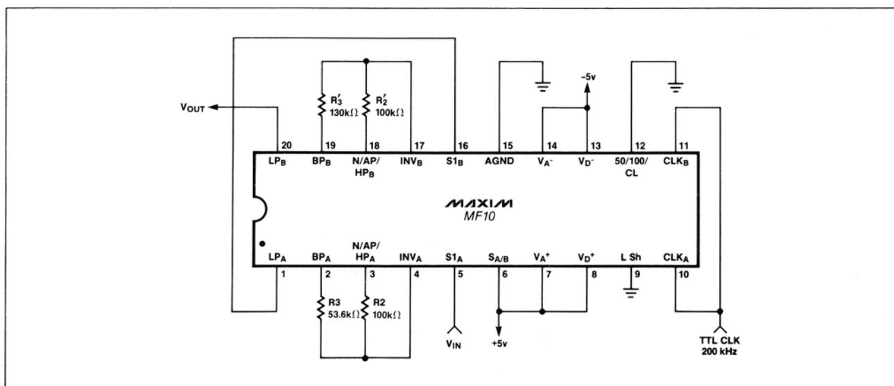
Figure 18. 4th Order, 2kHz Lowpass Butterworth Filter
