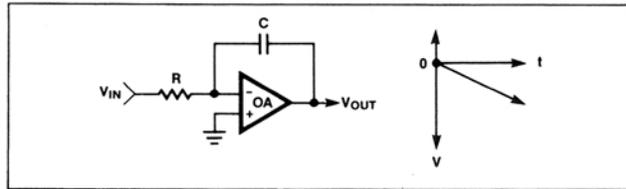
Figure 20. Typical RC integrator
