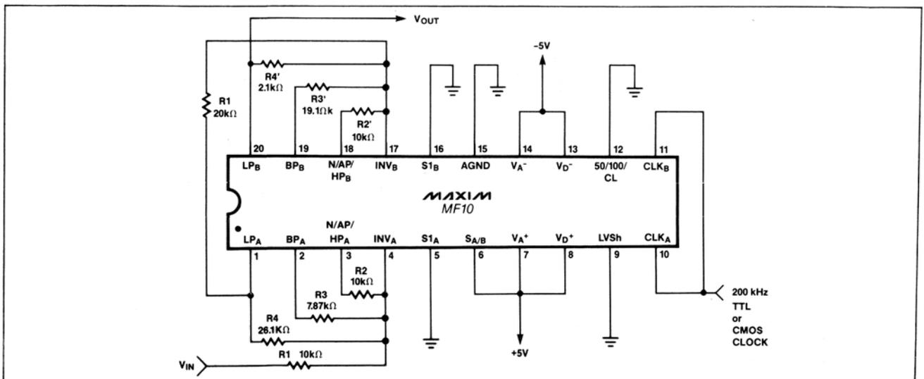
Figure 19. 4th Order Chebyshev 5kHz Lowpass Filter
