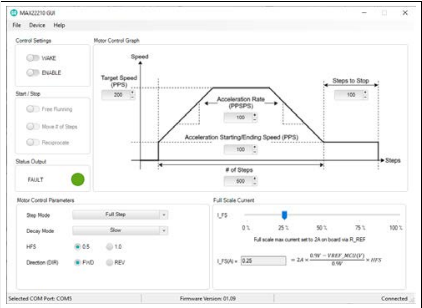
Figure 3. MAX22210 EV Kit GUI
