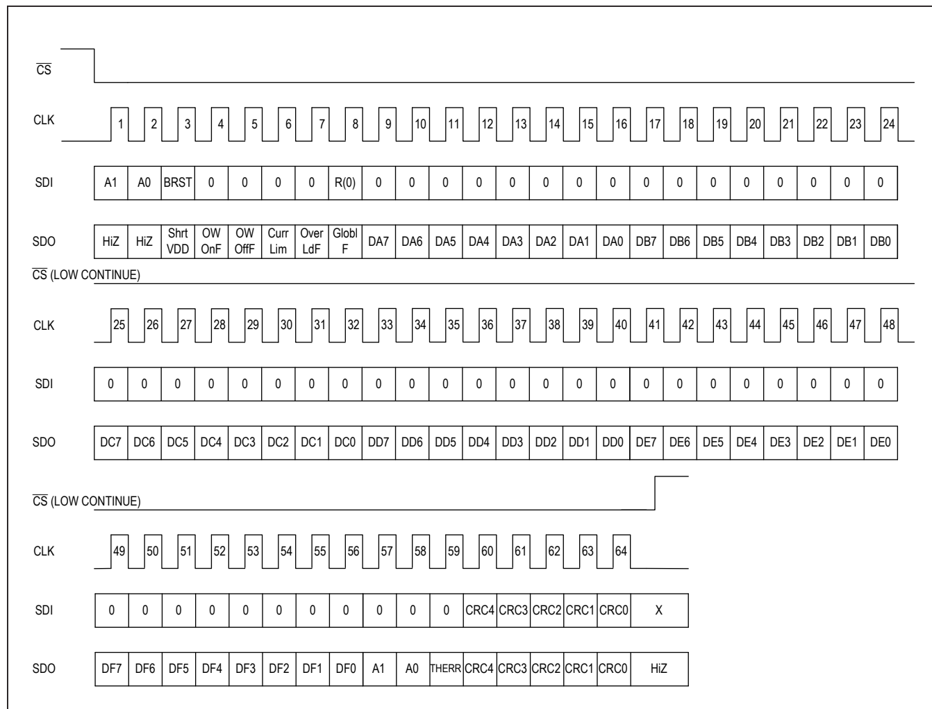
Figure 16. Addressed SPI Burst Read Command with CRC
