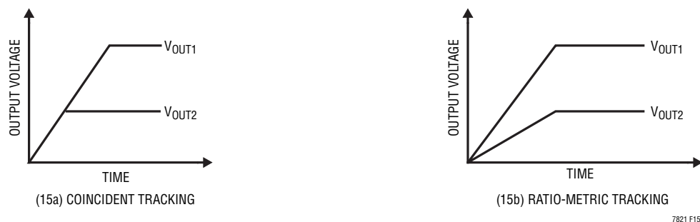
Figure 15. Two Different Methods of Output Voltage Tracking
