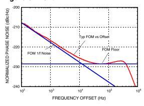
[1] Fractional Mode, 50 MHz Crystal, R=1, ~80 kHz Loop BW, (Loop filter values: C36 = 560pF, R26 = 680Ω, C35 =15nF, R27 & R28 = 1 kΩ, C37 & C38 = 270 pF) 2mA Charge Pump, -385 $\mu$ A Offset.
