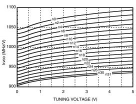
[1] Fractional Mode, 50 MHz Crystal, R=1, ~80 kHz Loop BW, Filter C36 = 560pF, R26 =  $680\Omega$ , C35 =15nF, R27 & R28 = 1 k $\Omega$ , C37 & C38 = 270 pF, 2mA Charge Pump, -385 $\mu$ A Offset.
