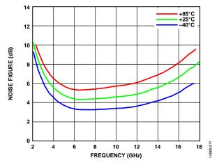
Figure 12. Noise Figure vs. Frequency for Various Temperatures
