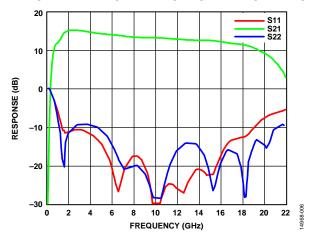
Figure 7. Response (Gain and Return Loss) vs. Frequency
