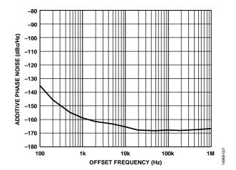
Figure 16. Additive Phase Noise vs. Offset Frequency, RF Frequency = 8 GHz, RF Input Power = 12 dBm (P<sub>SAT</sub>)
