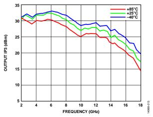
Figure 14. Output Third-Order Intercept (IP3) vs. Frequency for Various
