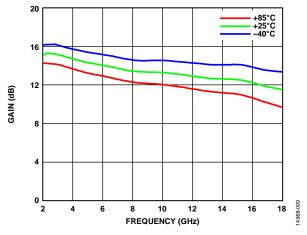
Figure 10. Gain vs. Frequency for Various Temperatures
