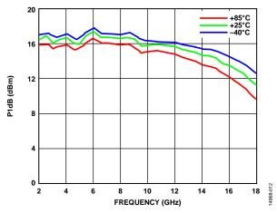
Figure 13. Power for 1 dB Compression (P1dB) vs. Frequency for Various Temperatures
