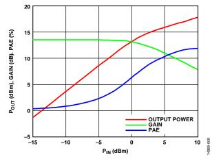
Figure 9. Output Power ( $P_{OUT}$ ), Gain, and Power Added Efficiency (PAE) vs. Input Power ( $P_{IN}$ )
