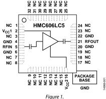
The HMC606LC5 provides 13.5 dB of small signal gain, 27 dBm output IP3, and 15 dBm of output power for 1 dB compression while requiring 64 mA from a 5.0 V supply. The input and output of the HMC606LC5 amplifier are internally matched to 50  $\Omega$ and are internally dc blocked.
