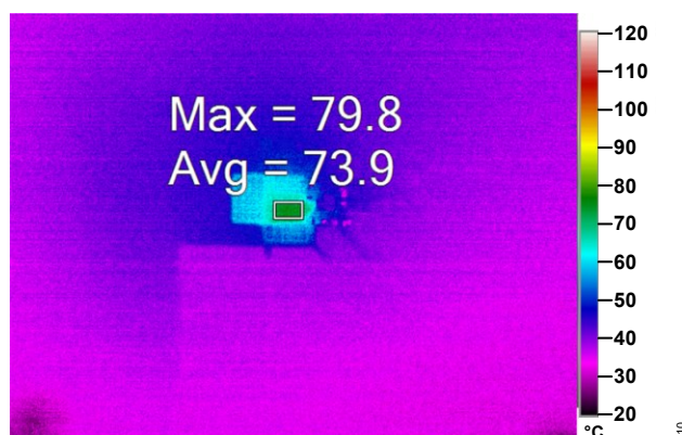
Figure 10. Thermal Image of Bottom Layer at 24V OUT , 5A I OUT , 500kHz. (Thermal Values are on Q1)
