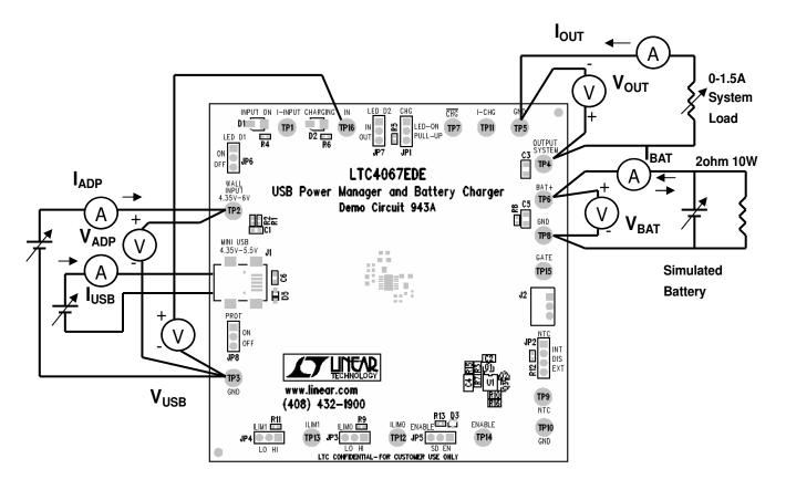
Figure 1. Proper Measurement Equipment Setup
