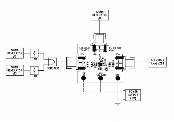
Figure 1. Proper Measurement Equipment Setup
