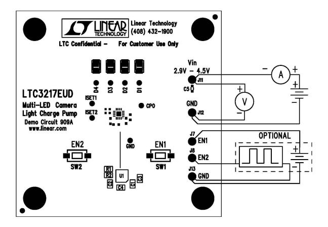
Figure 1. Proper Measurement Equipment Setup for DC909
