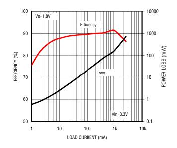
Figure 3. Efficiency and Loss vs Load Current (Burst Mode)
