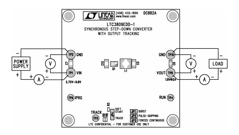
Figure 1. Proper Measurement Equipment Setup
