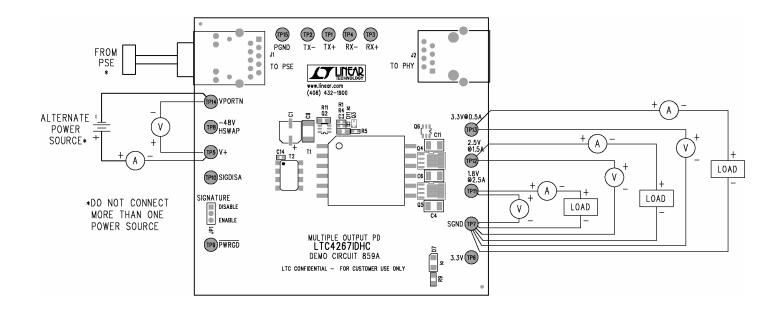
Figure 1. Proper Measurement Equipment Setup
