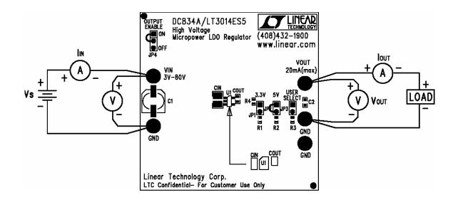
Figure1. Proper Measurement Equipment Setup
