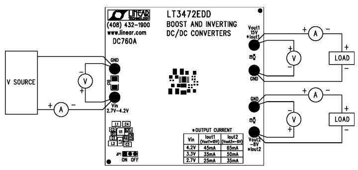
Figure 1. Proper Measurement Equipment Setup
