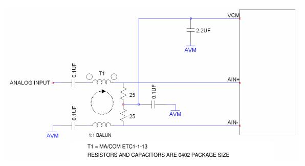
Figure 4. Analog Front End Circuit For 250MHz <  $A_{\mbox{\footnotesize{IN}}}$  < 500MHz
