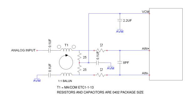
Figure 3. Analog Front End Circuit For 100MHz <  $A_{\mbox{\scriptsize IN}}$  < 250MHz
