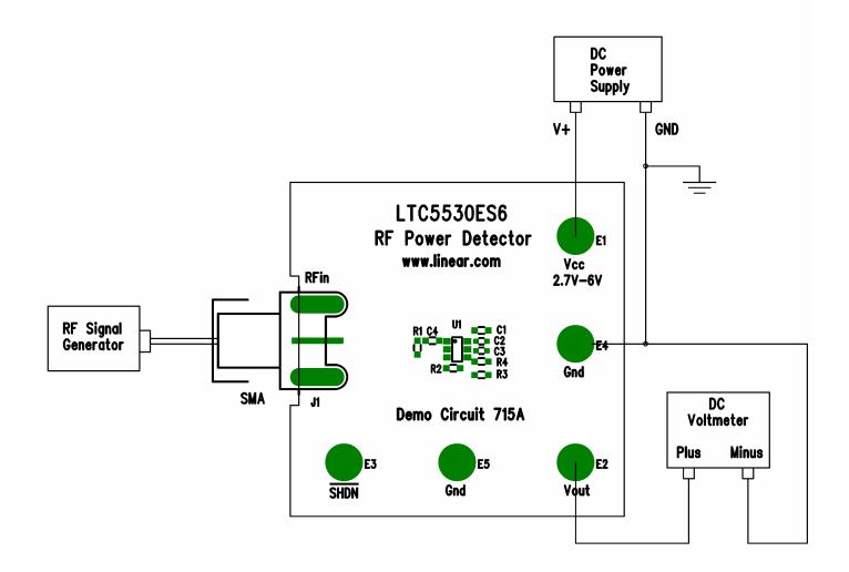
Figure 1. Proper Measurement Equipment Setup
