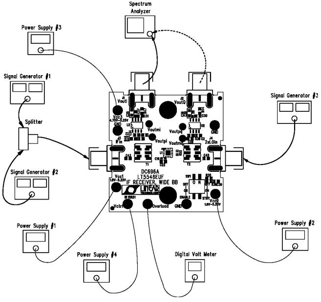
Figure 1. Test and Measurement Setup
