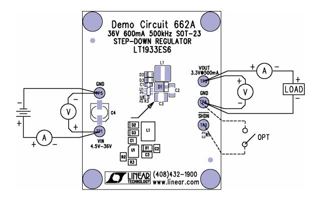
Figure 1. Proper Measurement Equipment Setup
