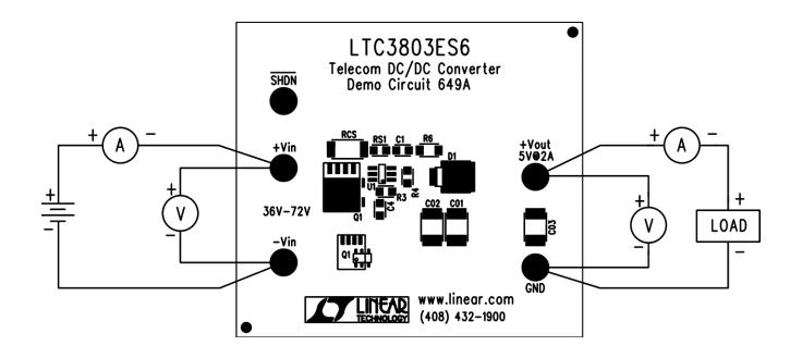
Figure 1. Proper Measurement Equipment Setup
