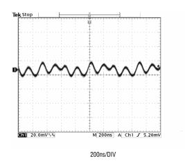
Figure 4. Typical Output Ripple ( $V_{IN} = 3.3V, V_{OUT} = 1.5V, I_{OUT} = 600mA$ )
