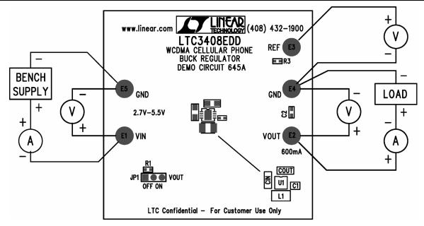
Figure 1. Proper Measurement Equipment Setup
