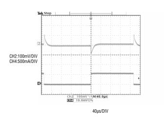
Figure 3. VOUT (100mV / Div) Transient Response for 0 to 600mA load Step.  $(V_{IN}=3.3V,\,V_{OUT}=1.2V)$
