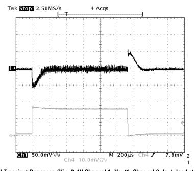
Figure 5. DC616A Load Transient Response (Vin=2.4V;Channel 1: Vout1; Channel 2: lout: load step from 0.2A to 2.25A)
