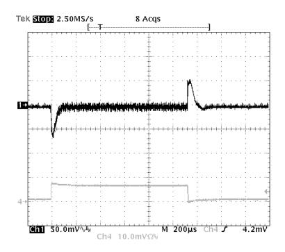
Figure 6. DC616B Load Transient Response (Vin=4.2V;Channel 1: Vout1; Channel 2: lout1: load step from 0.2A to 2A)
