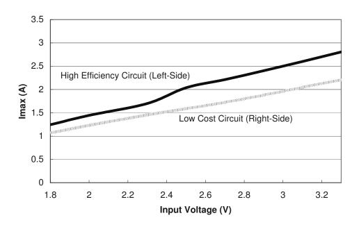
Figure 4. Maximum Output Current vs Input Voltage for 5V Output (DC616B)
