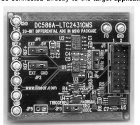
analog signals while using the DC590 USB Serial Controller board and supplied software to measure performance. The exposed ground planes allow proper grounding to prototype circuitry. After evaluating with Linear Technology's software, the digital signals can be connected to the end application's processor / controller for development of the serial interface.
