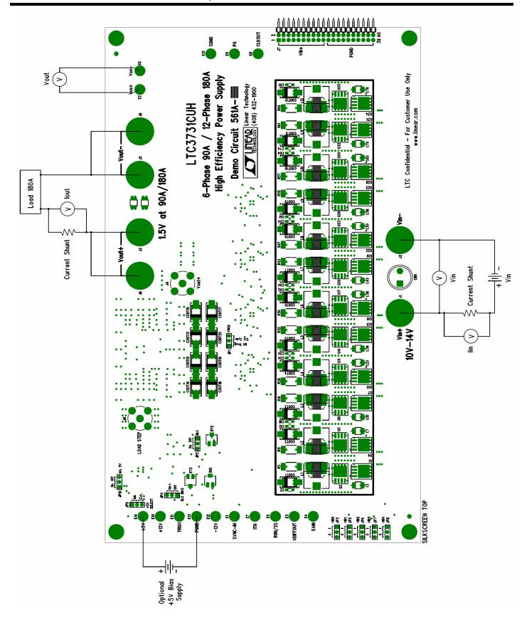
Figure 2. Proper Measurement Equipment Setup
