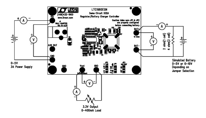
Figure 2. Proper Measurement Equipment Setup
