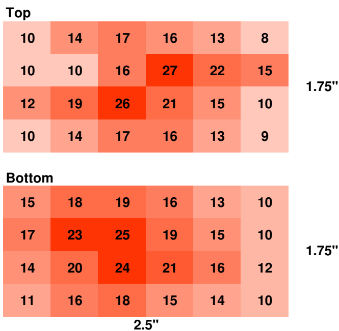
Figure 4. Temperature Gradient over the PCB while Dissipating 3W of Power.
