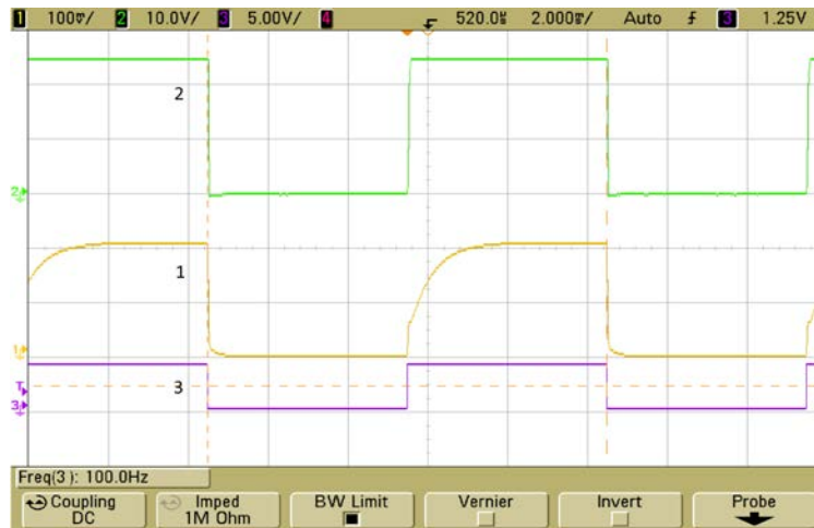
Figure 2. High Side Driver Voltage Waveforms. CH 1 Q2 Gate Voltage Relatively to Source (5V/DIV), CH 2 VOUT, CH 3 Sync Signal.
