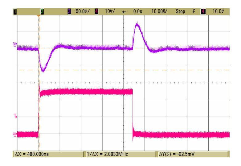
Figure 4. Load Step Response  $V_{IN}$  = 12V,  $V_{OUT}$  = 1.8V, 2.5A Load Step (0A <-> 2.5A)
